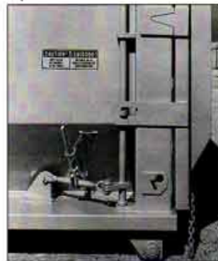
Heavy-duty ratchet latching mechanism aids water tight sealing of both sides of rear door
