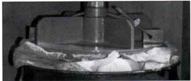
Standard platen adapts for compaction of materials into drum
